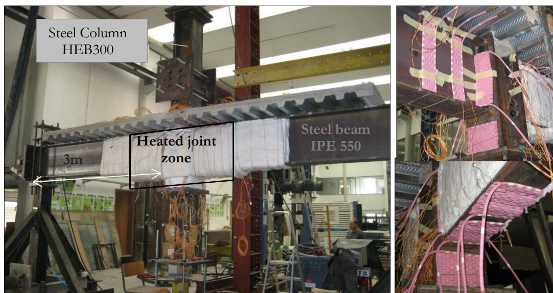
Figure 3.13: Heated connection zone using Ceramic Pad Heating elements, thermally insulated by rock-wool of density 128 kg/m 3 (tests 2 to 6)
