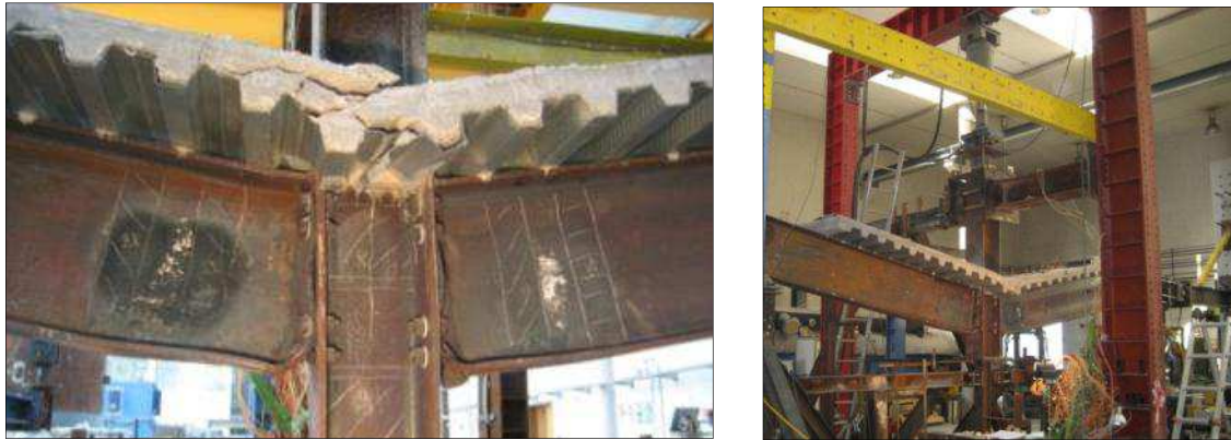
Figure 3.35: Final deformation of the tested structure (test 6)
