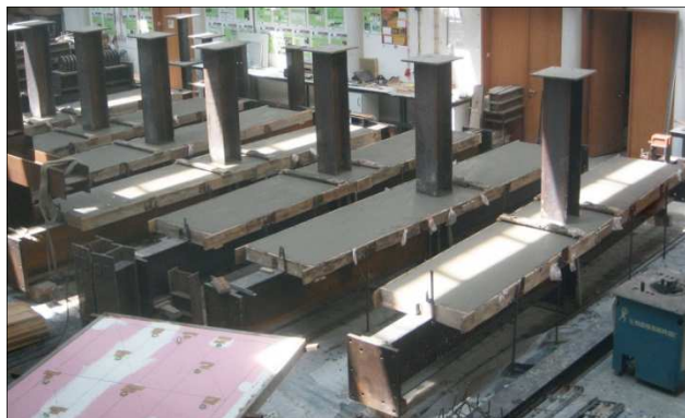
Figure 3.6: Specimens after the concreting of the composite slabs, at the floor level
