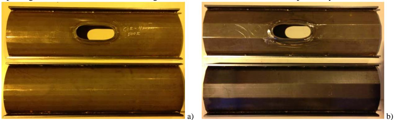
Fig. 4. a) Circular specimen with opening and Circular specimen; b) Polygonal specimen with opening and polygonal specimen
