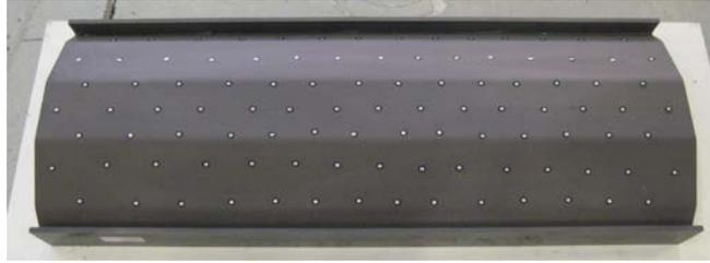
Fig. 2. Preparation of specimen for scanning geometric imperfections
