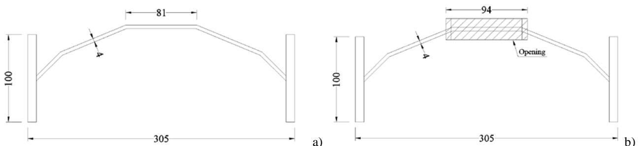
Fig. 1. a) Polygonal specimen; b) Polygonal specimen with opening
