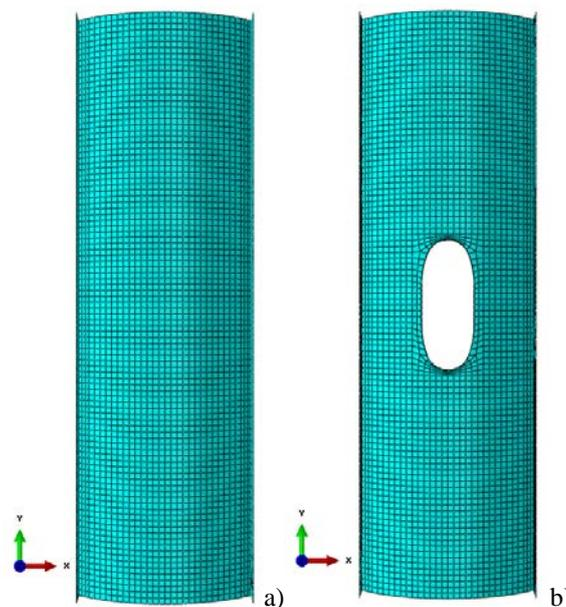
Fig. 3. a) FE mesh of the circular model; b) FE mesh of the circular model with the opening
