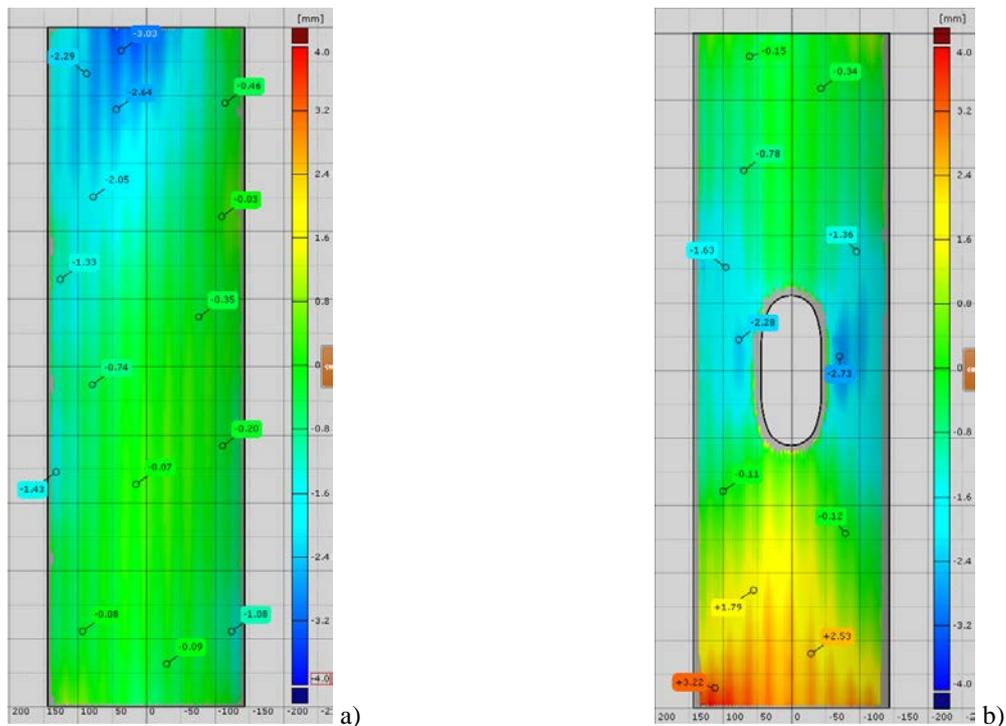
Fig. 6. Geometric imperfection from laser scanning: a) circular specimen; b) circular specimen with opening
