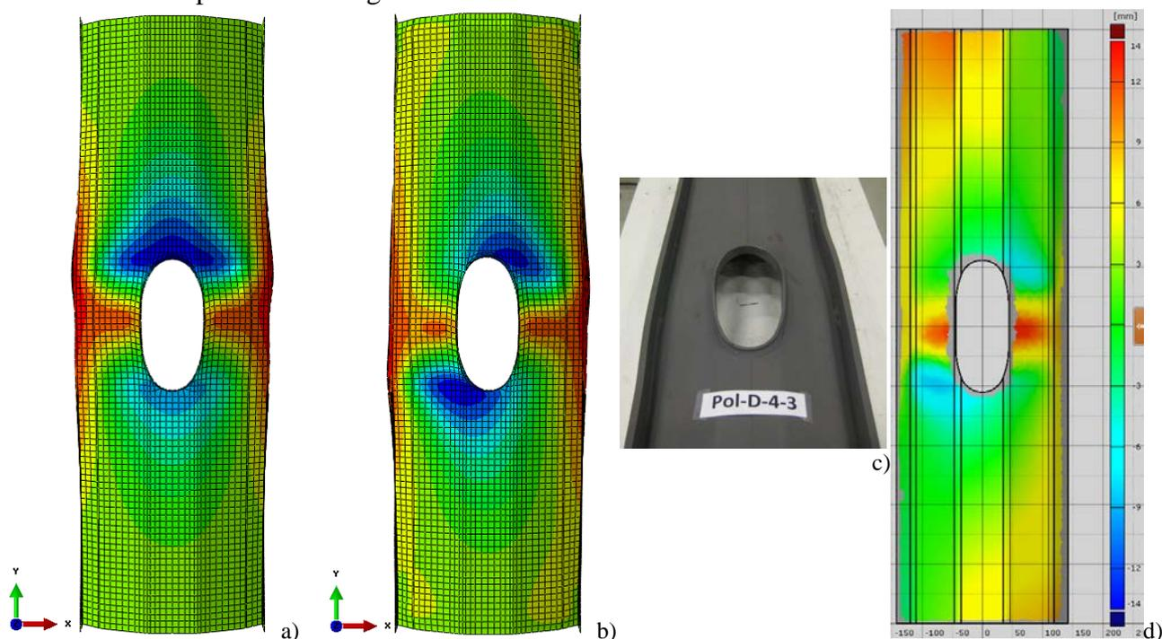
Fig. 8. Deformation of a) model with geometric imperfection according to Eurocode 3; b) model with geometric imperfection from laser scanning; c) specimen after the test; d) specimen after the test with laser scanning technology
