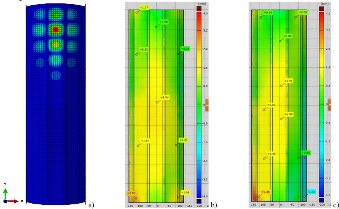
Fig. 7. a) buckling mode shape of polygonal model; b, c) geometric imperfection of specimens from laser scanning
